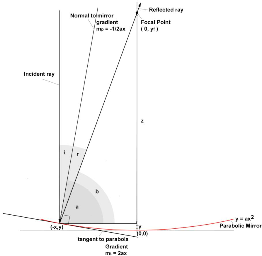
Angle of reflection ( $r$ ) equals the angle of incidence ( $i$ )
