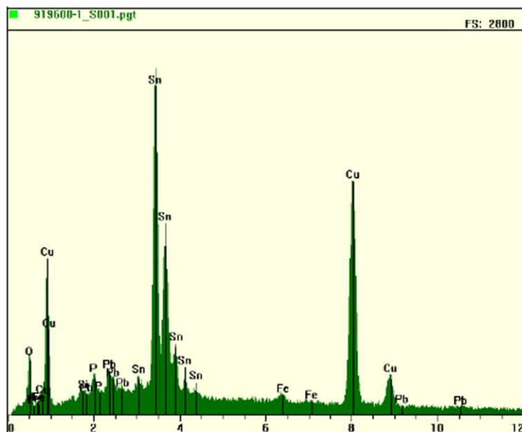
Figure 1: EDS spectrum of shiny surface
