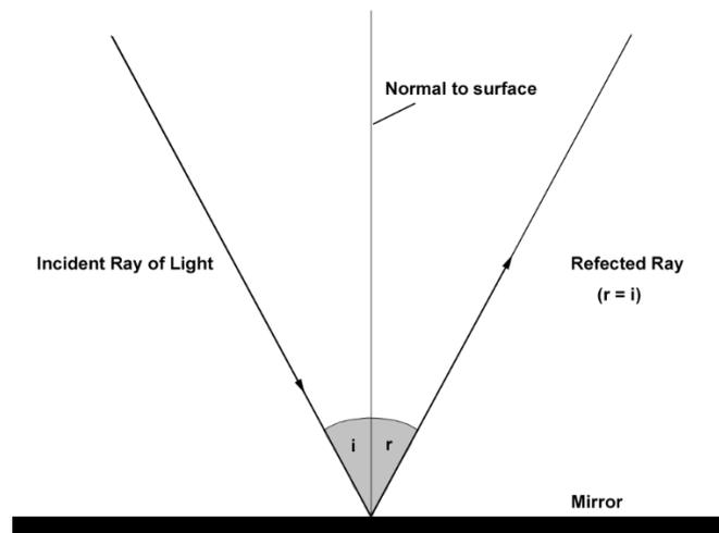
The angle of incidence (i) equals the angle of reflection (r). On a curved mirror surface the same principle applies and the angle of reflection can be determined by calculating the gradient of the tangent to the curve at the point of incidence on the mirror surface and then determining the normal to the tangent, that is the line that is perpendicular to the tangent.
