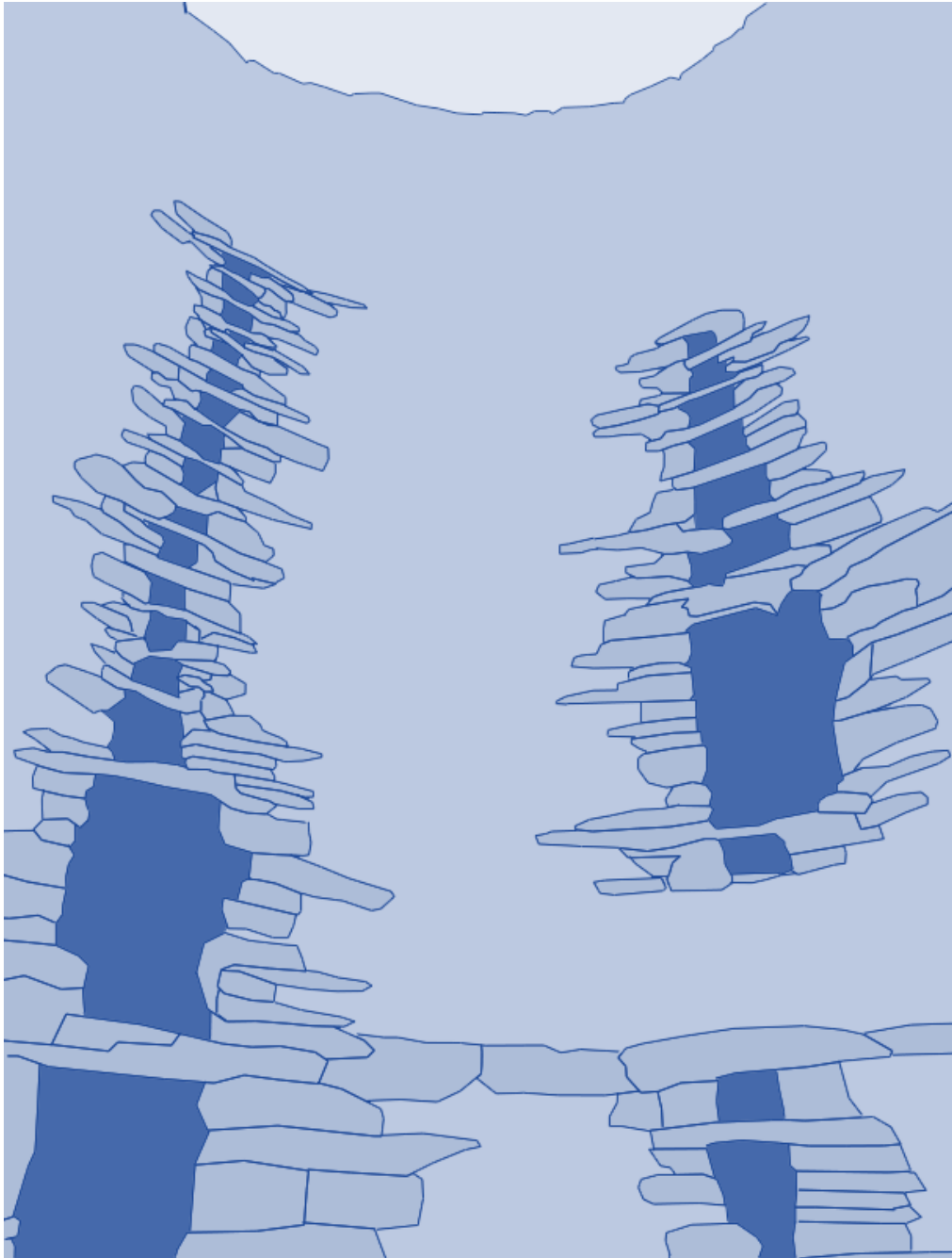
Figure 3 Mousa Broch lintelled openings in internal wall that allow light from the open roof into the spiral staircase
